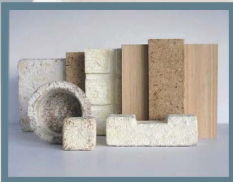
Mycology materials have only recently begun to be explored as an engineering material, and thus far research into their mechanical properties has been very limited. Mycelium is currently being commercially developed for packaging materials, insulation, structural insulating panels, and acoustical tiles.
